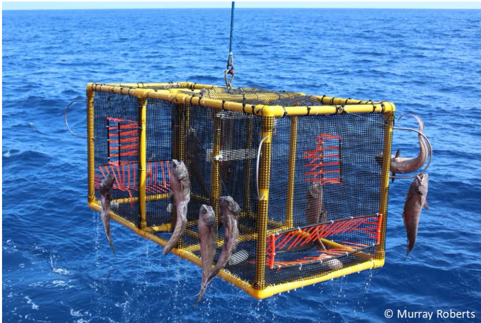
Figure 6.6.3.1.1 Recovery of the Baited Trap Lander, with rattail fish attached to fishhooks in- and outside the trap. The white HDPE bottles with holes and bait inside function as amphipod traps. (Image: Murray Roberts, University of Edinburgh).
