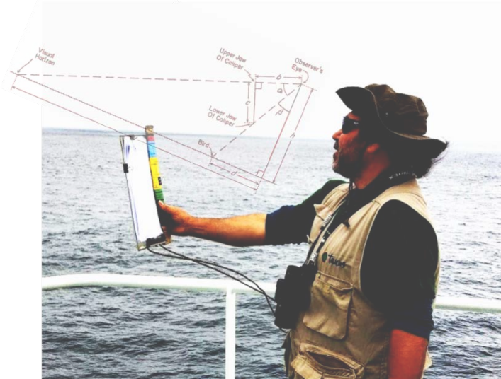
Figure 6.11.3.5 Joan Carles' demonstrates how to estimate the distance of a bird from the ship. The top of the ruler must be at the horizon, the arm outstretched and then he locates the position of the bird (d). The bandwidth will be bigger for the distances closer to the vessel and thinner for the distances further away. (Trigonometric figure modified from Heinemann 1981). (Image: seabird ecology team)
