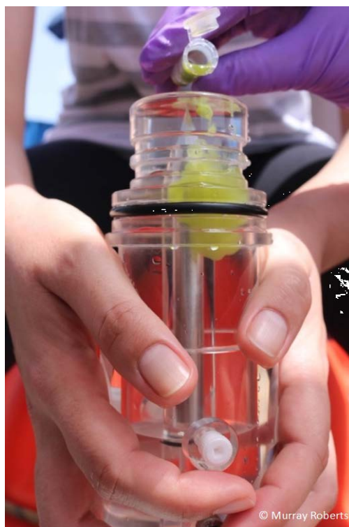
Figure 7.7.3.1 Addition of ^{13}\text{C} and ^{15}\text{N} isotopically labelled substrate (freeze-dried axenic algae Phaeodactylum tricornutum ) to the particle injector of the benthic respirometer lander. (Image: Murray Roberts, University of Edinburgh).
