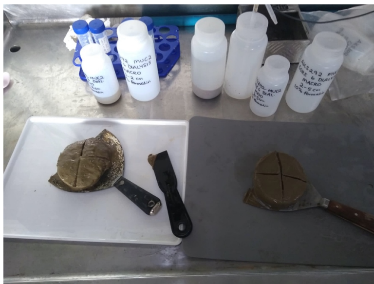
Figure 7.9.3.4 Example of core slicing. Core 6 was sliced into 0-2 cm (left) and 2-5 cm (right) horizons, each divided into a quarter for PLFA, a quarter for meiofauna, and half for macrofauna analysis. (Image: Danielle de Jonge).
