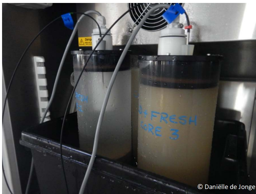
Figure 6.7.1.1 Ex situ sediment incubation set-up. Sediment cores sealed at the bottom are placed in black boxes with filtered seawater held at the experimental temperature that was maintained in the LMS incubators. During SCOC measurement intervals the cores were sealed at the top, gently stirred (white bars in image), and oxygen concentration measured using FireSting optodes (metal rods in image). (Image: Daniëlle de Jonge, HWU).
