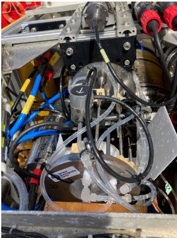
Figure 7.3.2.1 RoCSI inside the nose of Autosub6000. (Image: Susan Evans)
