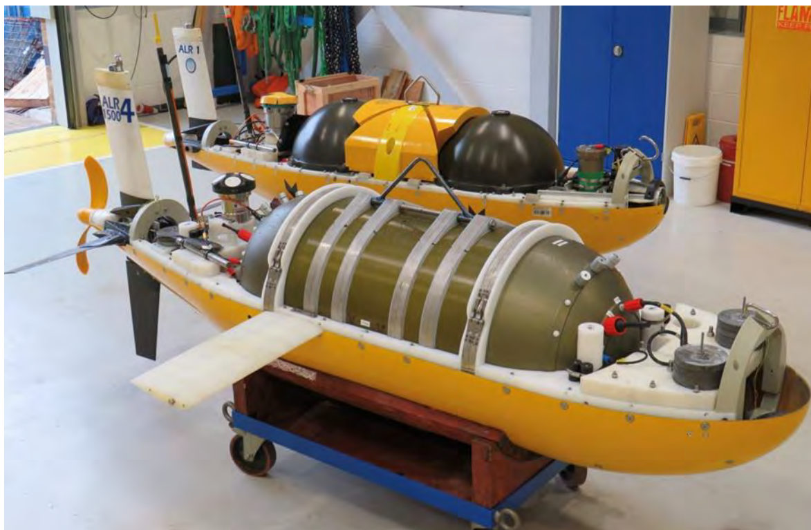
Figure 5.1: Autosub Long Range Variants, 6000m depth rated behind, 1500m in front
