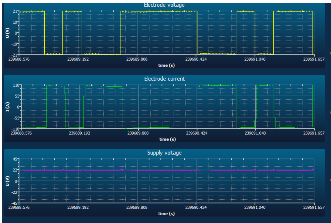
Figure 12: DASI.exe view, for monitoring output current and voltage status
