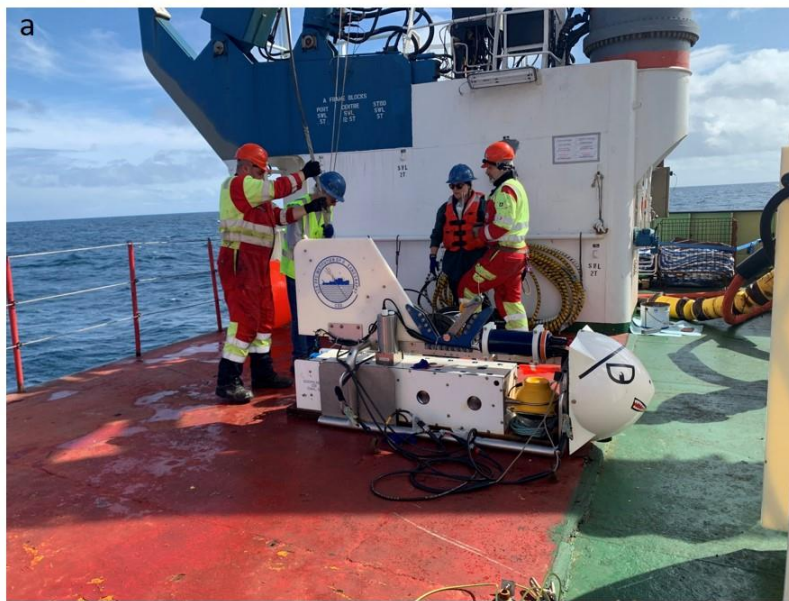
Figure 4: a) The LEM launcher getting ready to be deployed using the A frame. b) the same instrument being deployed.
