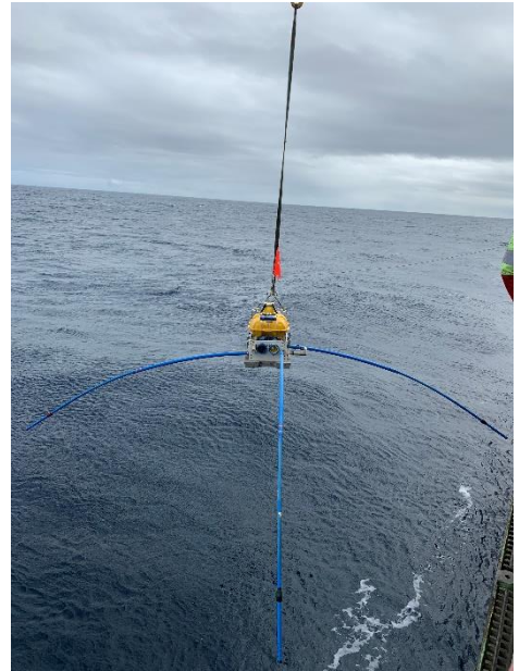
Figure 3: a) A Scripps OBI being prepared for deployment using the starboard crane. b) The same Scripps instrument is being deployed.
