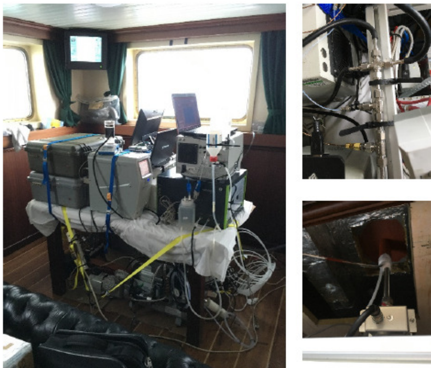
Figure 5. From left to right in the Chief Scientists Room on the A33: grey and green iDIRAC, measuring isoprene and DMS; grey nano Scanning Mobility Particle Spectrometer (SMPS) measuring particle size distributions 5-68nm; grey Condensation Particle Counter (CPC) total particle count >4nm; and black particle Size Magnifier (PSM) lowering cut of CPC between 1.4 and 3nm. The smaller photos show the sampling manifold for these instruments and the ¼ inch tube onnected connecting the manifold to the ¼ tube passing through the ship's port. Also in the photograph is the ¼ inch nylon exhaust tube for the CPC, SMPS and PSM.
